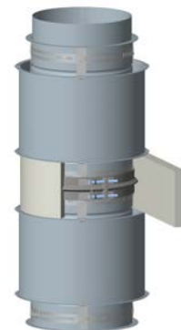
Figure 10 - Joint Assembly Step 5
