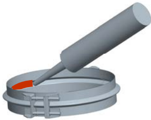
Figure 6 - Joint Assembly Step 1
