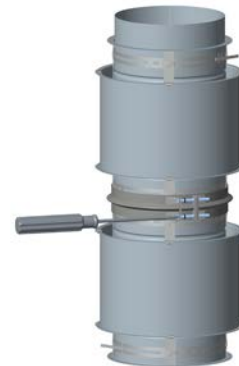
Figure 9 - Joint Assembly Step 4
