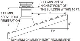
The chimney <u>shall</u> extend at least 3 feet above its point of contact with the roof, and at least 2 feet higher than any wall, roof or adjacent building within 10 feet of it. On a sloped roof, the roof itself will usually be the highest point. With steeper pitch, you will need to have more chimney above the roof deck.
