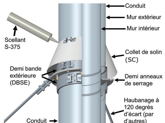
Schéma 66b - Haubanage installé
