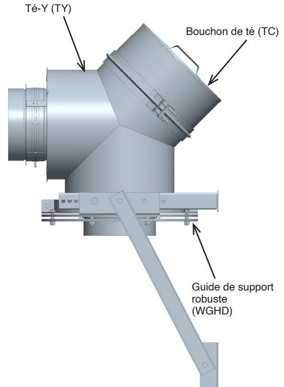
Schéma 95 - Installation of a Y-Tee (TY)
