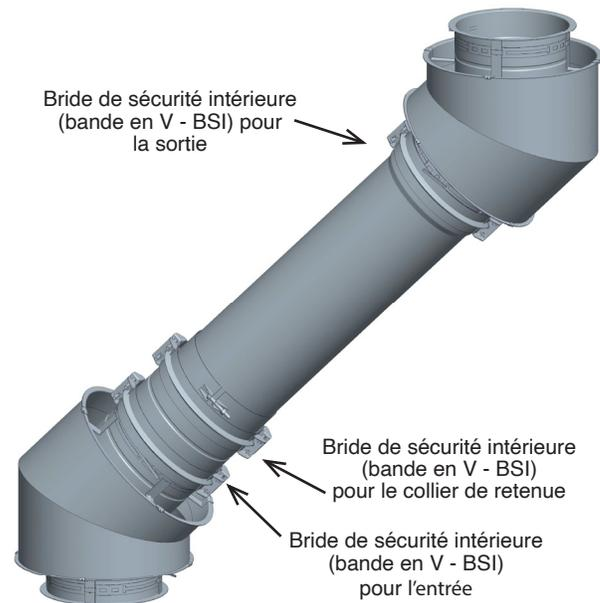
Figure 27 - Step 10-11 - Secure the Retaining Flanged Band
